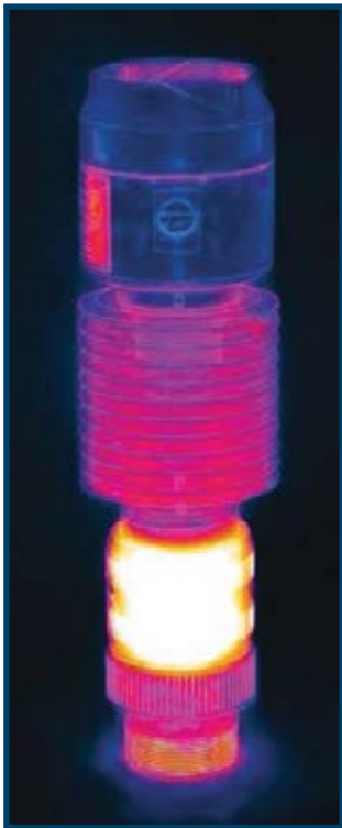
High Temperature Switch (Thermal Image)
